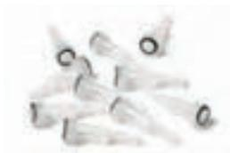
**Fig 2.2.** SpinTrap microspin columns.
