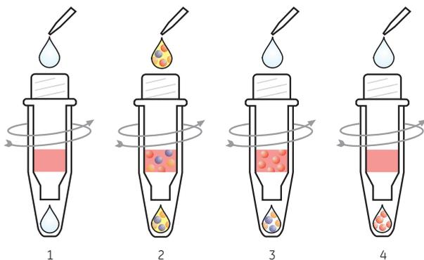
**Fig 3.40.** Purifying histidine-tagged proteins with His SpinTrap TALON is a simple four-stage procedure that can be performed in 10 min using a microcentrifuge: 1) After placing the column in a 2 ml microcentrifuge tube, equilibrate by adding binding buffer and centrifuge. 2) Add sample, centrifuge. 3) Wash with binding buffer, centrifuge. 4) Elute the target protein with elution by centrifugation
