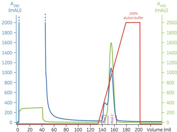
**Fig 3.25.** Purification of GFP-(His)<sub>6</sub> expressed in *E. coli* BL21 on HiScreen Ni FF. Indicated pools were analyzed by SDS-PAGE (Fig 3.26).
