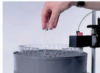
Fig 5.10. Typical procedures using ÄKTaprime plus. (A) Prepare the buffers. (B) Connect the column. (C) Prepare the fraction collector. (D) Load the sample.
