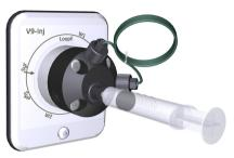
4 Load sample into the sample loop. To avoid sample loss due to siphoning, leave the syringe in the port until the sample has been injected onto the column during the run.
