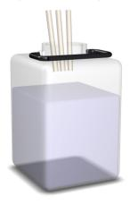
**Note:** If the tubing is too short, replace it with new tubing. Do not lengthen the tubing as this might cause obstruction of the tubing and flooding in the fraction collector chamber.
