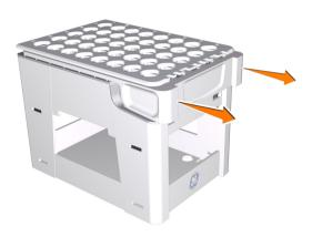
Place the tubes and deep well plates in the cassettes. Make sure that the deep well plates are rotated so that the well marked **A1** is positioned above the **A1** marking on the cassette.
