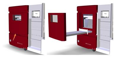
5.7 Prepare the built-in fraction collector
