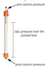
Fig. 7 Pre-column and post-column measurements.
