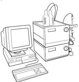
Components, such as the mixer, column and injection valve, are mounted to the right. Columns are snapped in place in column holders.
