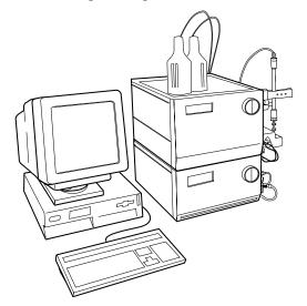
ÄKTAbasic consists of a compact separation unit and a personal computer running UNICORN $^{\text{m}}$  control system version 4.12 or higher. Fraction collectors are available as accessories.
