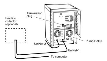
The UniNet-1 data communication cable is routed from the computer via the fraction collector, if used, to the rear of Pump P-900. UniNet-1 is terminated at Monitor UV-900 with a termination plug.
