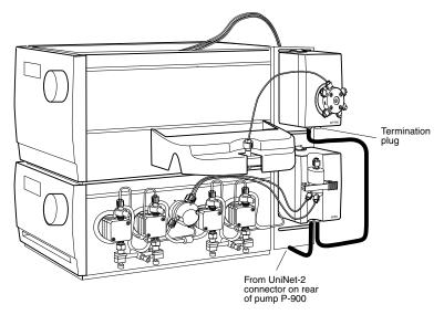
The UniNet-2 data communication cable which supplies the valves and mixer with control signals is routed from the rear of Pump P-900, and links components on the right side of the system. The cable is terminated at the injection valve, V1, with a termination plug.
