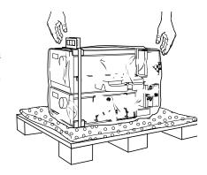
8 Detach the following items by cutting straps and removing red tape. Also remove the desiccant bags.
