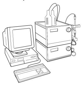
ÄKTAbasic consists of a compact separation unit and a personal computer running UNICORN software version 4.12 or higher. Fraction collectors are available as accessories.
