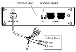
1 Connect the Mini-DIN cable connector to socket **Analog In** at AD-900.
