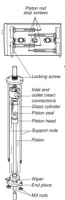
CAUTION! Do not push the piston at an angle to the cylinder and do not twist the piston.
