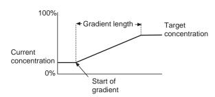
The gradient is run from current concentration to target concentration, over a set time or volume. The gradient can be set in any operating mode.
