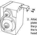
Attach the plate bracket to the pump using the two fillisterhead screws.
