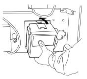
4. Push the pump towards the mounting plate as the figure shows. A click sound will indicate that the pump is locked in position.
