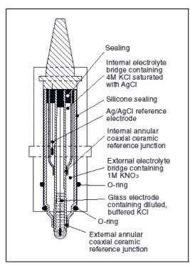
The pH electrode is of the sealed combination double junction type. It contains a sealed Ag/AgCl reference, which cannot be refilled, an internal electrolyte bridge of 4M KCl saturated with Ag/AgCl, an outer electrolyte bridge of 1M KNO<sub>3</sub>, an annular ceramic reference junction and a low profile pH membrane. The pH electrode is delivered with a transparent cover.
