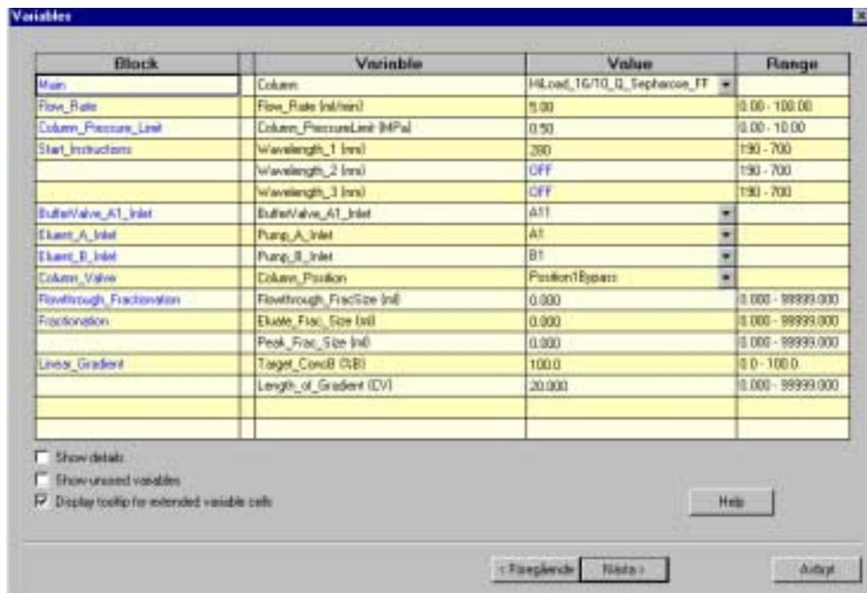
**Note:** When starting run no. 2 immediately after run no. 1 with the same method but, for example, a different flow rate, you simply: Click the Run button in System Control. Change the flow rate on the Variables page. Continue through the start protocol by clicking Next and then start the run. You do not need to change the method in the Method Editor.
