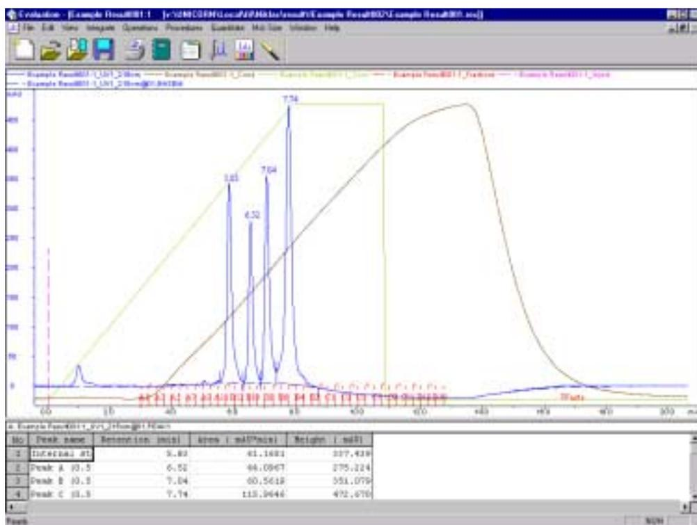
The result file from a run contains a complete record of the run, including method, system settings, curve data and run log.
