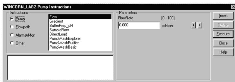
If, for example, you want to change the flow rate, select Pump and then Flow. Enter a new flow rate under Parameters and click Execute. The new flow rate will be used until the end of the run or until a new flow rate instruction is reached in the method.
