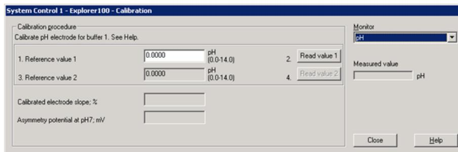
**Note:** Calibration can be performed with the electrode either within or outside the flow cell.
