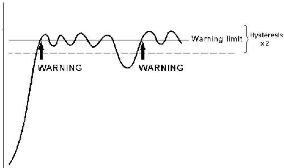
**Note:** Hysteresis is only relevant for warnings, since an alarm puts the system in **Pause** at the first alarm.
