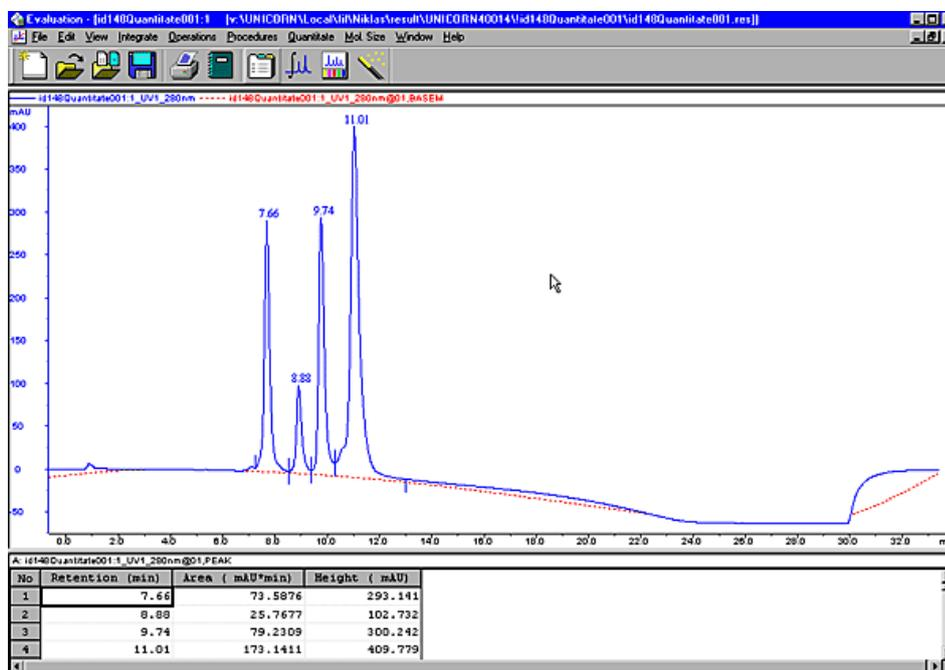
Note: The peak table is displayed underneath the active chromatogram. The start point and end point of each peak are marked by vertical marks, **drop-lines**.
